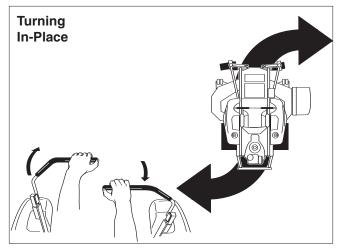
Figure 7. Turning in Place
